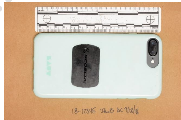
(D) Scale is in the same plane as the item (phone actual size).
